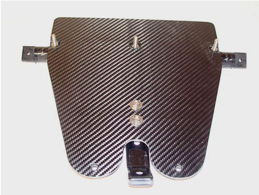
The 2007 Dreher carbon footstretcher board (shown with crossbar and carbon keel bracket for rake adjustment) for Sykes is used in all Sykes multiple-seat boats, except the M29 2x.
