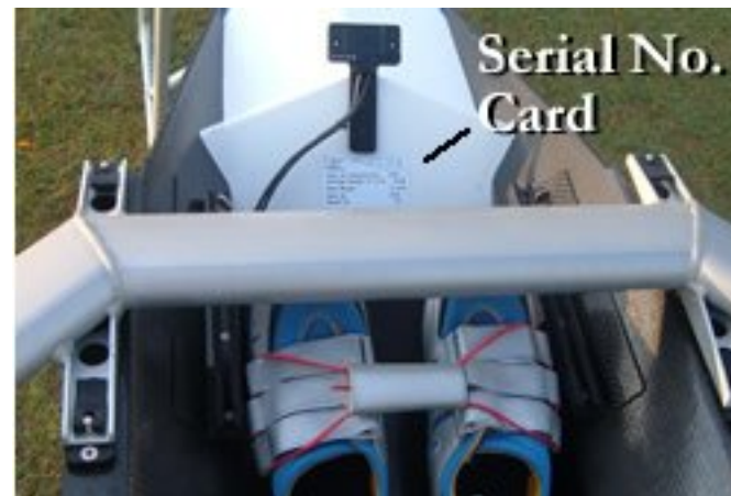
The serial number card is located astern the stroke seat's footstretcher in all boats except stern-coxed boats, in which case it is under the splash-guard.
