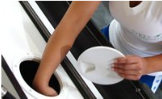
The wingnuts on the bow end are accessible through the porthole in the seat deck and slightly forward.
